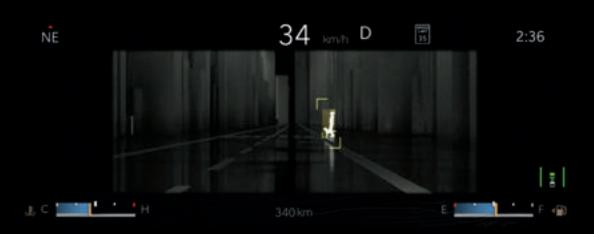
NIGHT-VISION CAMERA<sup>19</sup> An infrared eye mounted on the front grille detects pedestrians and animals crossing the vehicle's pathway. The driver is notified in time to take appropriate action. Available.
