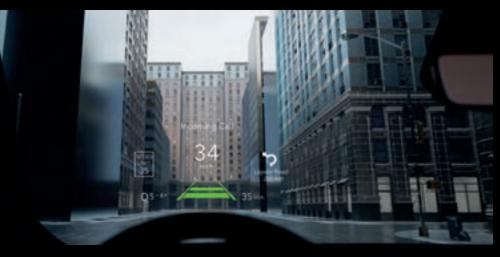
HEAD-UP DISPLAY WINDSHIELD Drivers can maintain focus on the road ahead with the help of this full-colour, transparent windshield display. Driving cluster data is projected onto a safe viewing area on the windshield in front of the driver. Available.
